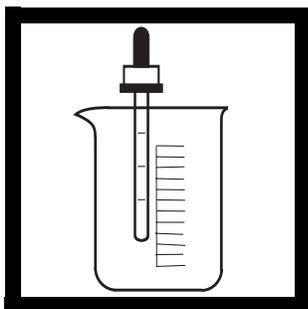
2. Rinse the glass dropper with sample water. Fill glass dropper to the 0.5-mL mark with sample water.
