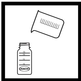
1. Fill the mixing bottle to the 23-mL mark with the sample water.
