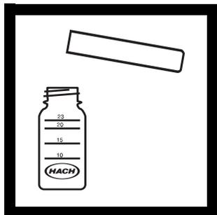
11. Pour the contents of the tube into a square mixing bottle.
