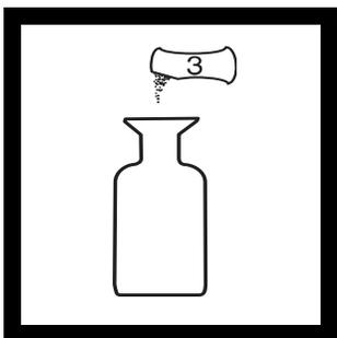
8. Remove the stopper and add the contents of one Dissolved Oxygen 3 Reagent Powder Pillow. Stopper the bottle carefully to avoid trapping air bubbles. If bubbles become trapped, discard the sample and repeat the test.
