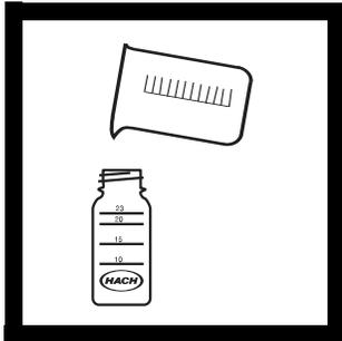
1. Fill the square mixing bottle to the 20-mL mark with sample water.
