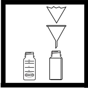
4. Place the funnel in the other square mixing bottle. Insert a folded filter paper into the funnel.
