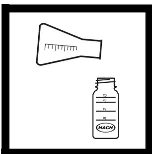
8. Return the sample to the square mixing bottle. Add deionized water rinsings from the flask to return the volume to 20 mL. Swirl to mix. Proceed with a total phosphate ascorbic acid test in the expected concentration range.
