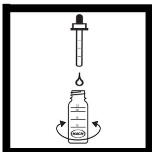
4. Add Sodium Thiosulfate Standard Solution one drop at a time to the mixing bottle. Count each drop. Swirl to mix after each drop. Add drops until the sample becomes colorless. It should take 10 drops of 0.0109 N Sodium Thiosulfate Standard Solution for the titration end point.
