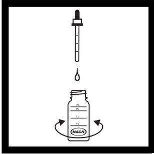
5. Add Sulfuric Acid Standard Solution one drop at a time. Count each drop. Swirl the mixing bottle after each drop is added. Add drops until the sample turns pink.
