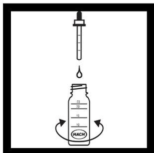
12. Add Sodium Thiosulfate Standard Solution one drop at a time to the mixing bottle. Count each drop. Swirl to mix after each drop. Add drops until the sample becomes colorless.
