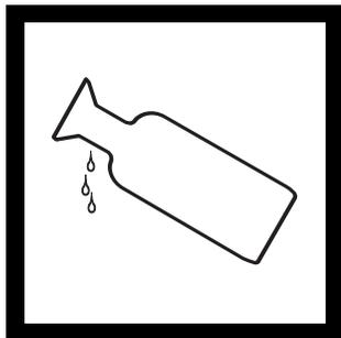
1. Use the prepared sample left from *step 10* of the High Range Test. Pour off the contents of the Dissolved Oxygen bottle until the level reaches the 30-mL mark on the bottle.
