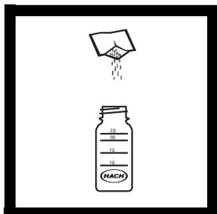
4. Add the contents of one PhosVer<sup>®</sup> 3 Phosphate Reagent Powder Pillow to the bottle containing 20 ml of digested sample water.
