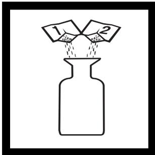
3. Remove the stopper and add the contents of one Dissolved Oxygen 1 Reagent Powder Pillow and one Dissolved Oxygen 2 Reagent Powder Pillow. Stopper the bottle carefully to avoid trapping air bubbles. If bubbles become trapped, discard the sample and repeat the test.
