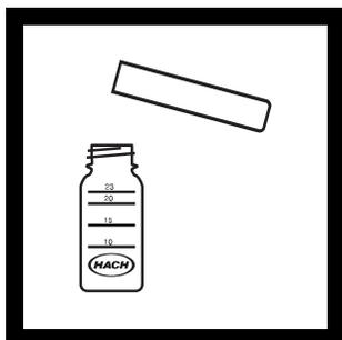
2. Pour the contents of the tube into a square mixing bottle.
