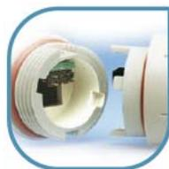
To install the new sensor, line up the tabs and 8 pins of the sensor to the instrument body. Twist ribbed collar back on to keep waterproof rating and secure sensor. The O-rings should create a watertight seal and provide some resistance when twisting.
